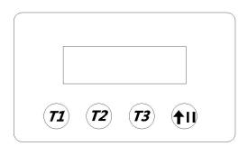
**T1 button** (1 min button): press this button, the clamping plate automatically clamps the canister, and finish appointed 1 minute mixing.
