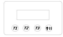
**T1 button** (**1 min button**) : press this button, the clamping plate automatically clamps the canister, and finish appointed 1 minute mixing.
