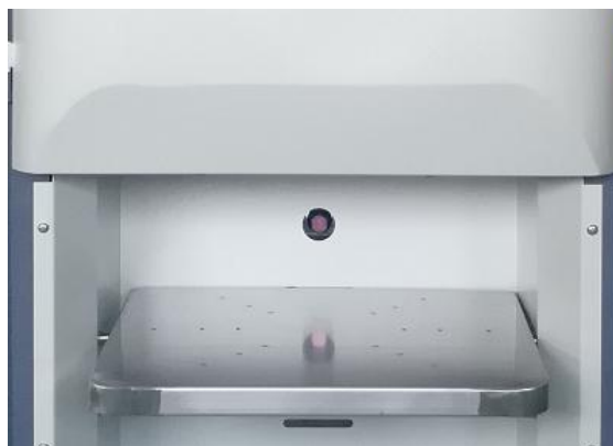
Can sensor, give alarm if there no can.
