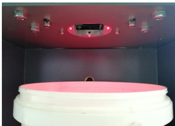
Laser light, help to locate paint can.
