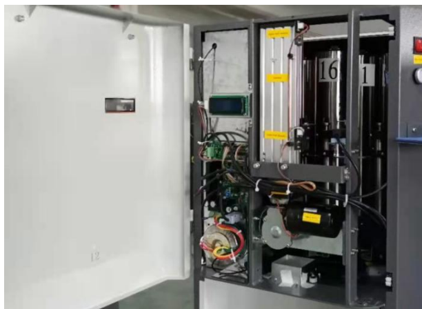
Mainboard and electrical structure install in the front, convenient to maintain.
