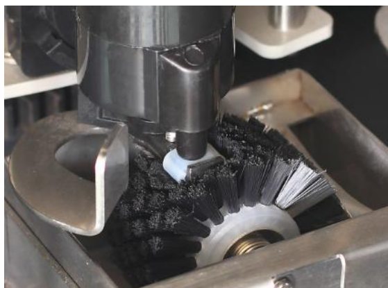
Rolling brush, clean nozzles automatically.
