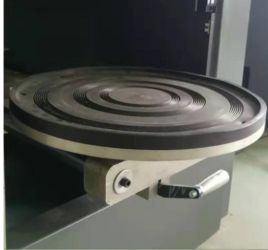
Extractable lower clamping plate , load and unload can conveniently
